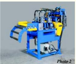
5 roll straightener 2 hydraulic 10 ton punches air press with punch tooling servo roll feed hydraulic shear Capacity: 16 gauge x 48" Sped 30 to 80 fpm\*
